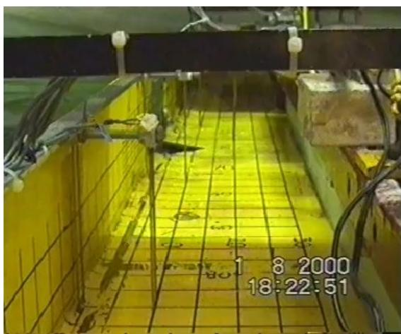
**Figure 22:** Typical Ro-Ro vessel set up for flooding capsize with water on deck
