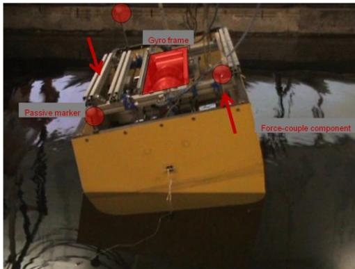
**Figure 16:** Experiments – Arrangements for forced oscillations of a free-floating RoPax section
