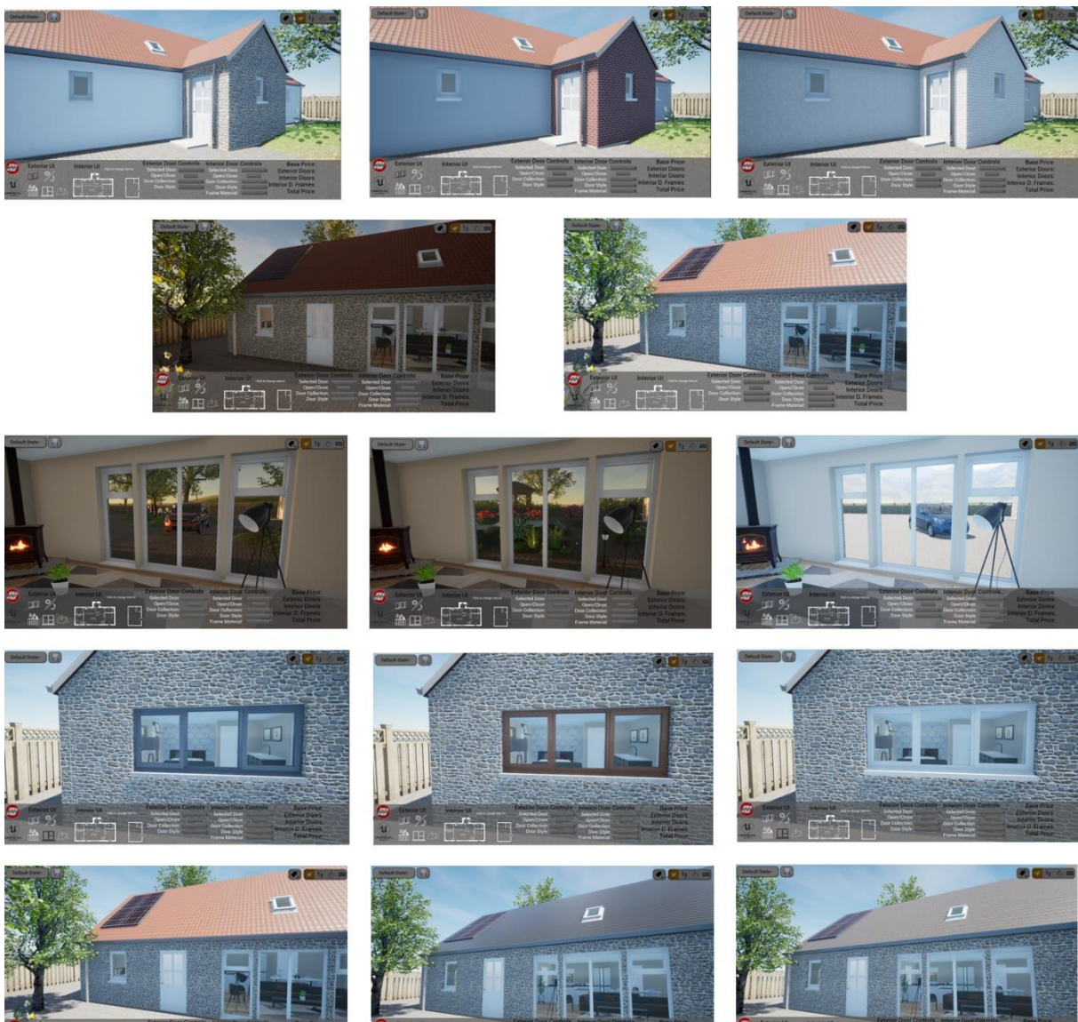
Fig. 8 House Configurator. Exterior variables examples. Rows from top to bottom: (1) Façade Styles; (2) Lighting Scenarios; (3) Garden options; (4) Window materials; (5) Roof variables.
