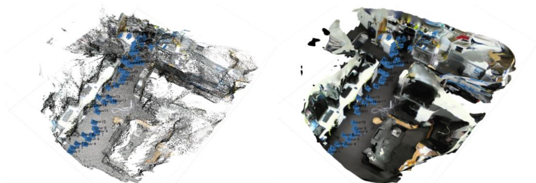
Fig. 7: 3D model of verification space (Point cloud display (left), polygon display with texture (right))
