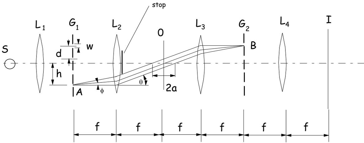
Figure 1: Optical setup
