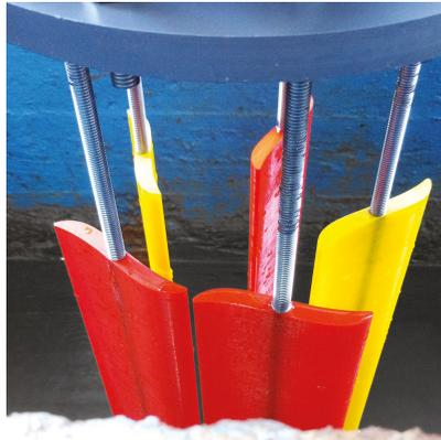
**Figure 23.** 3D printed blades installed on the prototype.
