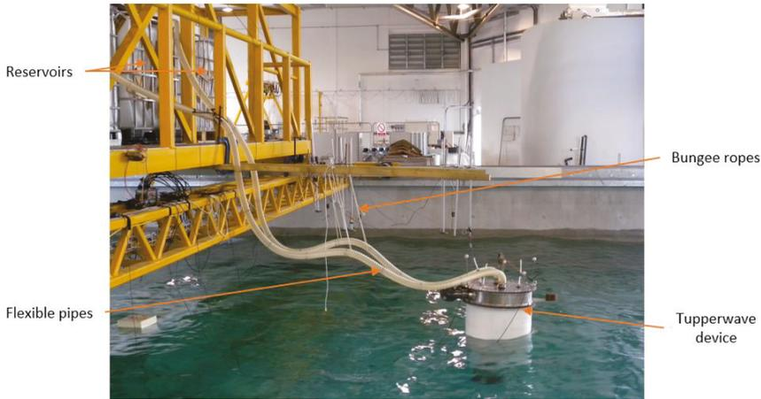
Figure 5. Physical model of the Tupperwave device.
