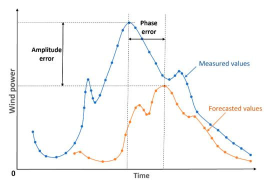
Figure 3. Amplitude and phase errors of wind power forecasting.
