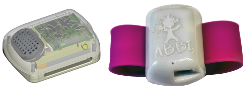
Figure 5. A render and photo of our audible beacon prototype.
