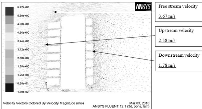
Fig. 8 Velocity vectors representation – cross-sectional view
