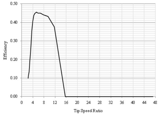
Fig. 9 Plot of tip speed ratio vs. efficiency.
