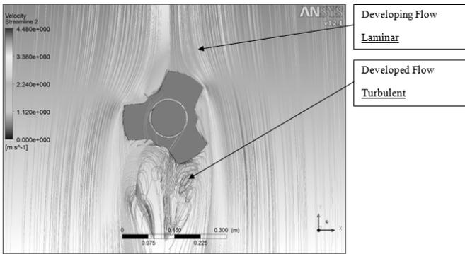
Fig. 7 Velocity streamlines distribution – top view
