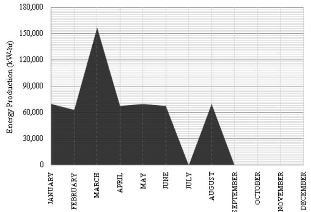
Fig. 11 Monthly energy production from the WinWind 3.0MW horizontal axis wind turbine
