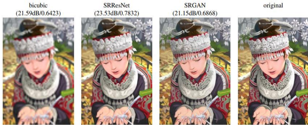
Fig. 7. [34] From left to right, image is reconstructed by bicubic interpolation, deep residual network (SRResNet) measured by MSE, SRGAN optimize more sensitive to human perception, original image. Corresponding PSNR and SSIM are provided on top.
