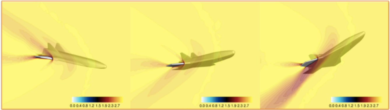
Fig. 11. Mach 3.0 contours for \alpha = -10 -deg (left), \alpha = 7.5 -deg (centre), \alpha = 25 -deg (right) for Y = 4.263 -metres
