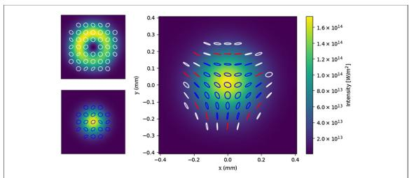
**Figure 3.** Poincaré polarization distribution downstream of the afterburner. The Delta undulators are set to have orthogonal circular polarizations. The electrons are bunched at the second harmonic of the first undulator and the fundamental of the second undulator. The radiation emitted in each Delta undulator is plotted (left) along with the combined field from both undulators (right).
