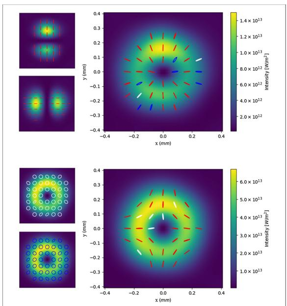
**Figure 2.** Simulation of cylindrical vector polarizations. The electrons are bunched at the second harmonic of the Delta undulators to give orthogonal linear (top) and circular (bottom) polarization. The radiation polarization emitted from each Delta undulator is plotted schematically on the (left) two plots and the combined field simulated from both undulators on the (right) plot. Red, blue and white lines correspond to linear, right-circular and left-circular polarization respectively.
