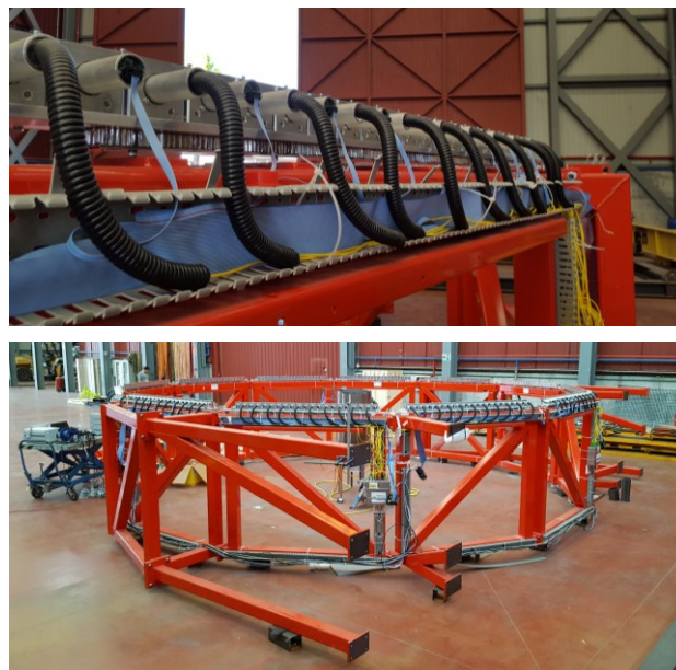
Fig.2. Detail (top) of an alignment plate showing mechanically supported fibers (yellow/black) to the transmit modules, and the preamplifier PCBs with ribbon cables (blue). Custom optical kinematic mounts, the ‘ring’ (red) during on-site build and fiber 1:21 splitter boxes are also shown (bottom). Visible in the center of the ring (bottom) is a propane gas-burner to provide deterministic placement and concentration CO 2 for phantom imaging tests.
