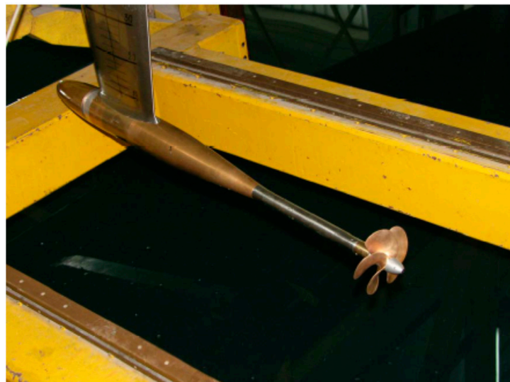
Figure 10. CTO Towing tank open water test set-up.
