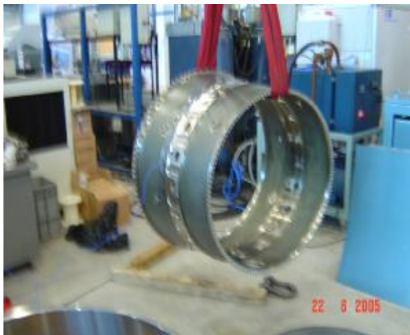
(a). A freely suspended engine-casing for modal test.
