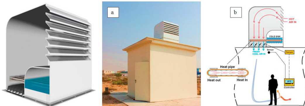
Fig. 1. (a) A roof mounted windcatcher with heat transfer devices (b) schematic diagram of the windcatcher operation.
