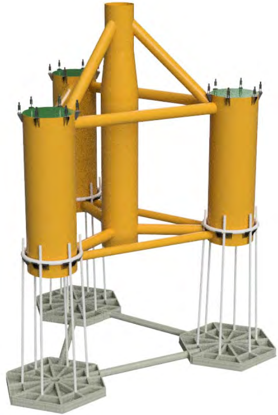
Figure 15 Isometric view of drop keel foundation concept in operational configuration
