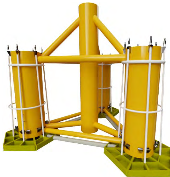
Figure 16 Isometric view of drop keel foundation concept in assembly/transit configuration
