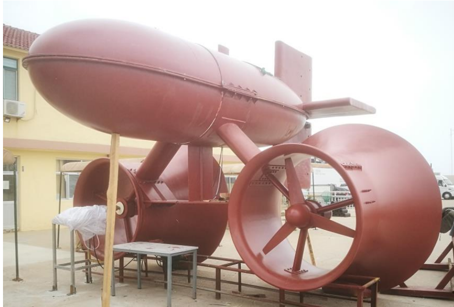
Fig.31 Photograph of the full-scaled submerged tidal current device
