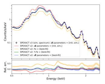
**Figure 4.** EPIC MOS 2 simulated spectrum of a 3T plasma with  $kT_{\rm mean} = 0.7$  keV, using SPEXACT v3. For comparison, we show the same model calculated using SPEXACT v2 (red). Then, we progressively fix the Fe (orange), Y (green), and eventually  $kT_{\rm mean}$ ,  $kT_{\rm up}$ , and  $kT_{\rm low}$  (blue) to their a posteriori best-fitting SPEXACT v2 values. The residuals of such models with respect to the input simulated spectrum are shown in the bottom panel.
