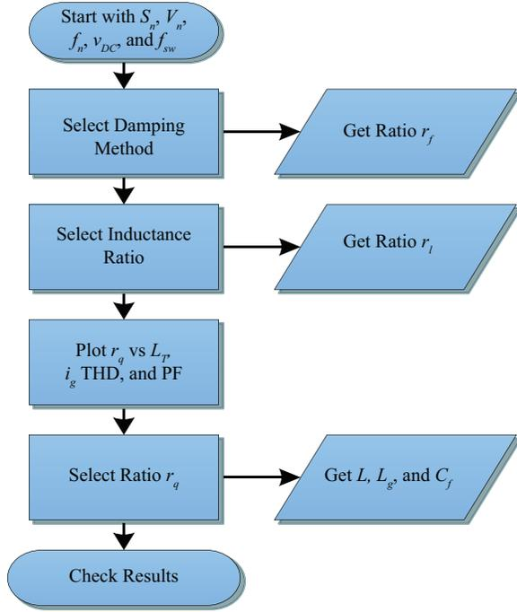
Fig. 6. Design flow for the LCL-filter.
