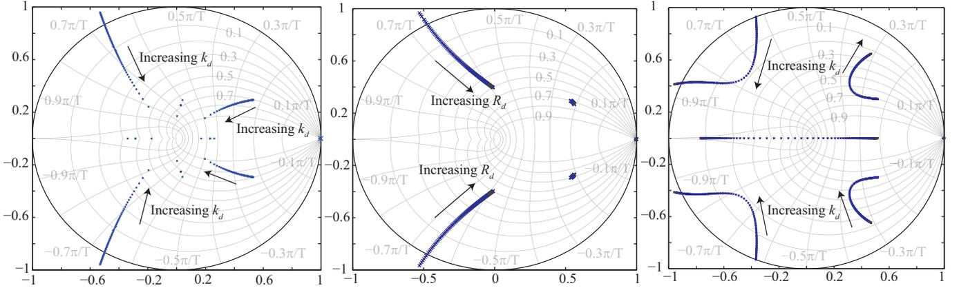
Fig. 8. Root locus in the  $z$ -plane by varying a)  $k_d$  for active damping with capacitor current feedback, b)  $R_d$  for passive damping and c)  $k_d$  for active damping with the lead-lag network.
