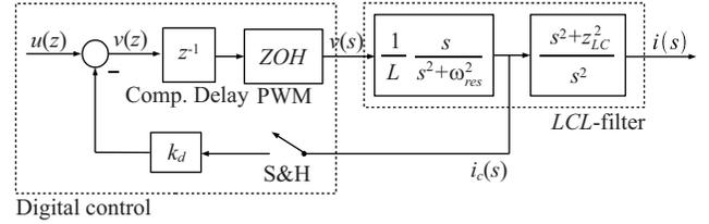
Fig. 5. Digital implementation of the capacitor current feedback.
