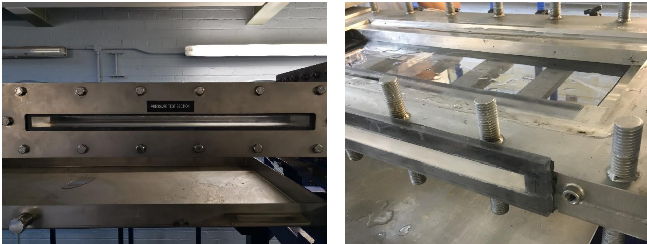
Figure 3: Side window in the measuring section of the FTFC
