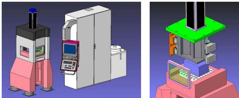
The machine is designed for minimum sizes using the state of the art design solutions to ensure a desktop type configuration. Integration with other micro-forming systems being developed in this project has also been considered in the frame of a multi-system integrated manufacturing facility as planned in the MASMICRO project. For that consideration, a high level control strategy has been planned, that will lead to an uniform integration and operation of several different, miniaturised machines.
