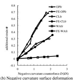
Figure 5. Relation curves of counterforce-additional strain at outer flange of side columns top
