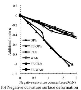
Figure 7. Relation curves of counterforce-additional strain at upper flange of middle-column-end of frame beam
