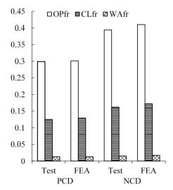
Figure 6. Comparison of variation rates of additional strain at outer flange of side column top Both the mudsill and infilled wallboard decelerates the variation of additional strain on the side column top. By contrast, the effect of infilled wallboard to the variation-rate of additional strain at outer flange of side columns top is greater than that of the mudsill.
