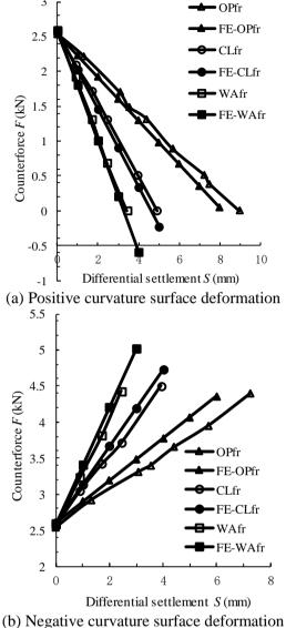
Figure 3. Relation curves of differential settlement- counterforce of side columns
