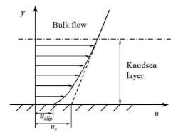
Fig. 1: Schematic diagram showing the actual microscopic slip  $(u_{slip})$  and the predicted macroscopic slip  $(u_s)$  based on Navier-Stokes equation with macro slip boundary condition within the Knudsen layer for Kramers' problem.
