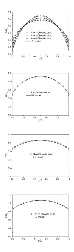
Fig. 8: The velocity profiles of the planar Poiseuille flows. Our LB model results are compared with the solutions of the linearised Boltzmann equation given by Ohwada *et al.* [47]. p-10
