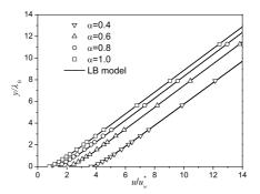
Fig. 4: The velocity profiles of the Kramers' problem with different tangential momentum accommodation coefficients.  $u_w^* = (2/\sqrt{\pi})\lambda_0 u_w/L$ . The symbols are the data from Loyalka *et al* [45].
