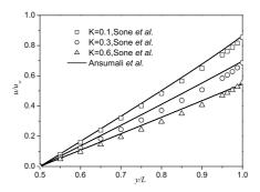
Fig. 6: The velocity profiles of the planar Couette flows. Our LB model results are compared with the analytical solutions given by Ansumali *et al.* [31]. The results of the linearised Boltzmann equation are given by Sone *et al.* [46].
