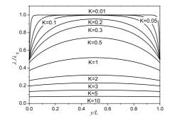
Fig. 2: The local mean free path profiles between two plates.
