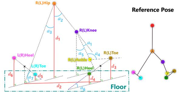
**Fig. 2:** Visual representation of distances  $d_i$  and angles  $a_i$  that are used to define gait parameters in Table I. ‘x’ denotes the 3D position at a segment centroid of two relevant joints represented by the same colour-coded cycles as in Fig. 1. Note that in this figure, the camera is placed at the subject’s right side. Thus R (right) ankle is captured while L (left) ankle is only tracked when the camera is placed on the left side.
