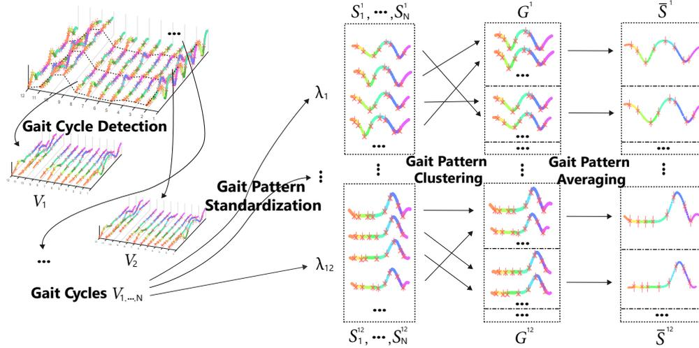
**Fig. 5:** Proposed gait pattern extraction, showing steps from left to right: extraction of gait parameter curves  $V^{\lambda_i}$  via gait cycle detection, then standardizing to  $S^z$  (Step1), clustering to  $G^z$  (Step2) and averaging as  $\bar{S}^z$  (Step3).
