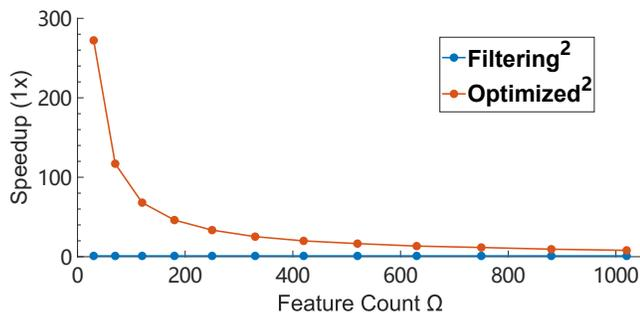
**Fig. 12:** Computation performance (1x times of baseline) of the proposed feature extraction methods: the base line computation time is measured using the filtering method with 1020 feature candidate pairs.
