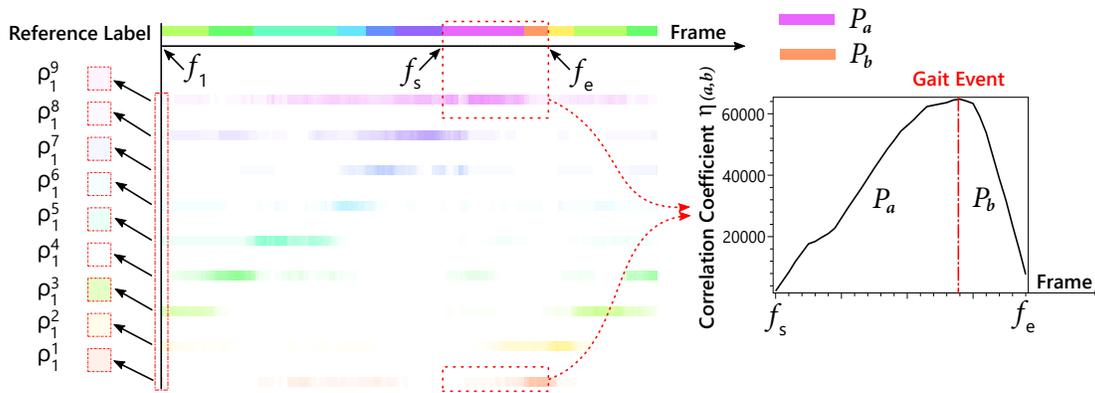
**Fig. 8:** Class probability representation in a complete gait cycle and correlation coefficient for adjacent gait phase periods. Unique color is assigned to each gait phase label where low transparency means low probability of the label occurrence at specified frame.
