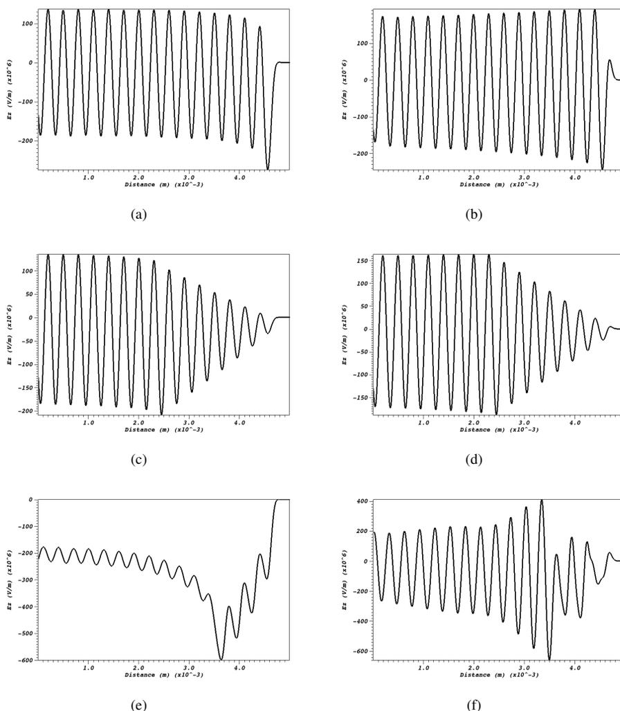
Figure 2: a,b) Single bunch of 8 nC, c,d) eight bunches with 1 nC each and separated by  $\lambda_p$ , e,f) eight bunches with 1 nC each and separated by  $\lambda_p/2$  at the first time step and after 100 mm propagation into the plasma, respectively.
