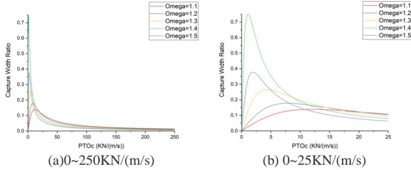
Fig. 4. Curve of capture width ratio versus PTO damping coefficient
