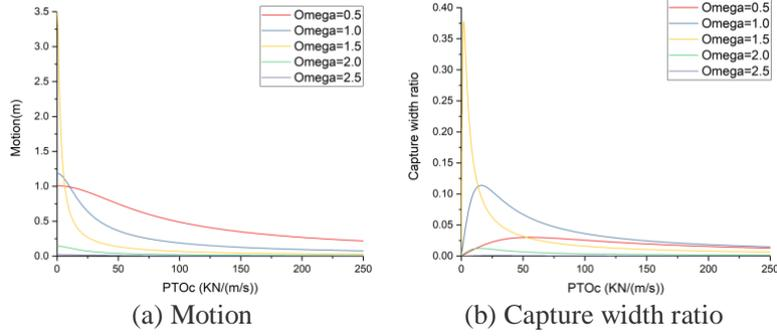
Fig. 3. Curve of dynamic characteristics versus PTO damping coefficient
