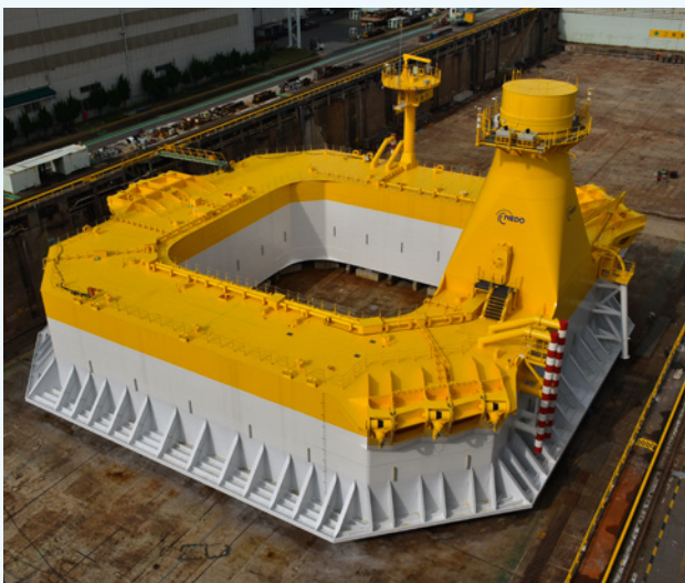
Figure 4: Ideol's 3 MW Damping Pool barge design, Kitakyushu, Japan (Source: Ole.stobbe.offshore)
