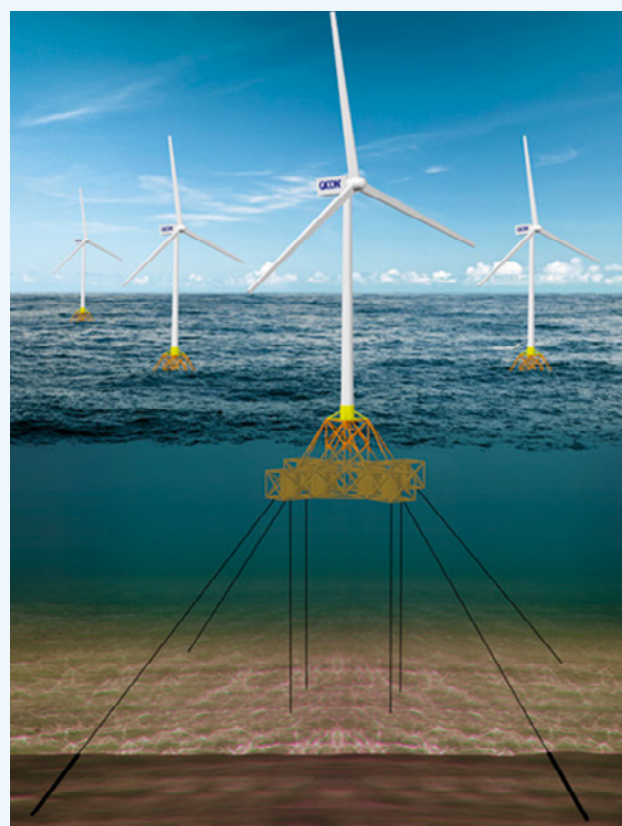
Figure 7: TLP concept from Gicon SOF (Source: GICON GmbH)
