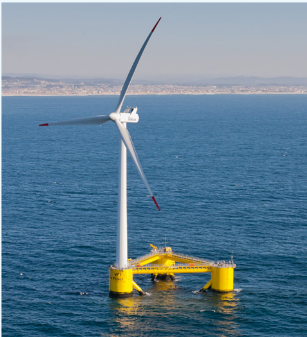
Figure 3: WindFloat 2 MW prototype design from Principle Power, Aguçadoura, Portugal (Source: Untrakdrover)
