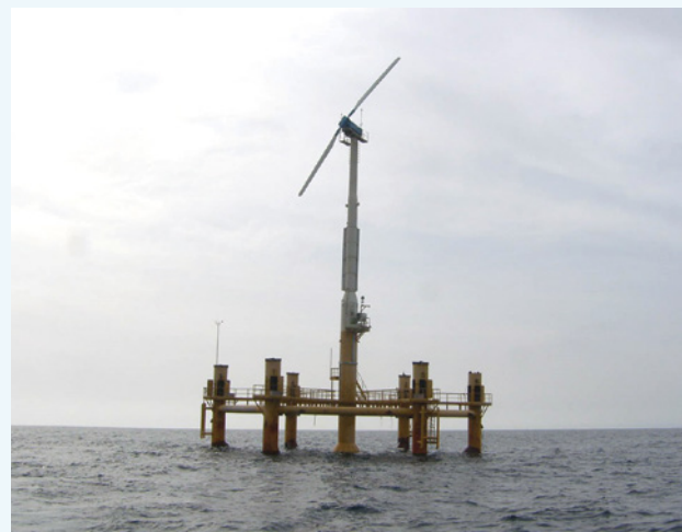
Figure 6: Blue H Technologies' concept, deployed off Brindisi, Italy (Source: Green Storm 7)
