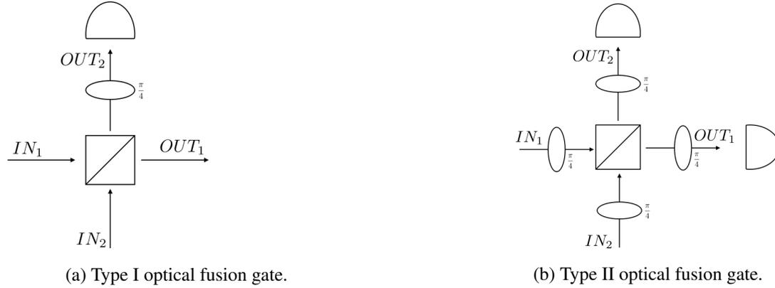
Figure 5: The two types of optical fusion gates using a polarising beam splitter and detectors in the polarisation  $|H, V\rangle$  basis. Both work post-selectively to entangle the inputs  $IN_1$  and  $IN_2$ .
