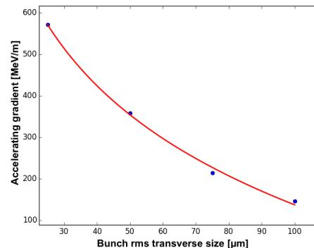
Figure 5: Dependence of average accelerating gradient for particles in the tail of the bunch on bunch radius, for a plasma density of  $3 \times 10^{22} \text{ m}^{-3}$ . The red line shows a least-squares fit to  $\log(\text{const.}/\sigma_r)$ , the expected relation from the linear theory for a cigar-shaped bunch [8].
