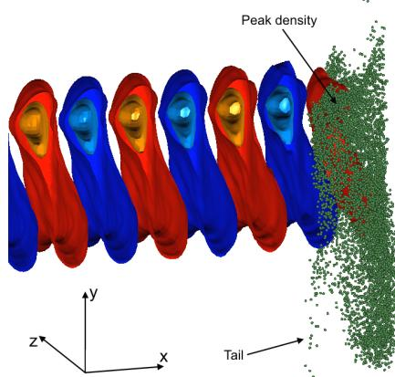
Figure 7: Isosurface plot of longitudinal electric field and bunch macroparticles for 3D simulation of a realistic CLARA-FE bunch. The isosurfaces are clipped in the x-y plane for visibility. The longitudinal coordinate is x.
