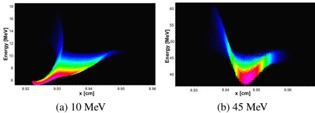
Figure 3: 2D histogram of the longitudinal phase space after 9 cm for bunches with initial energies of 10 MeV and 45 MeV. The colour scale corresponds to the sum of the weights of the macroparticles in the histogram bin.
