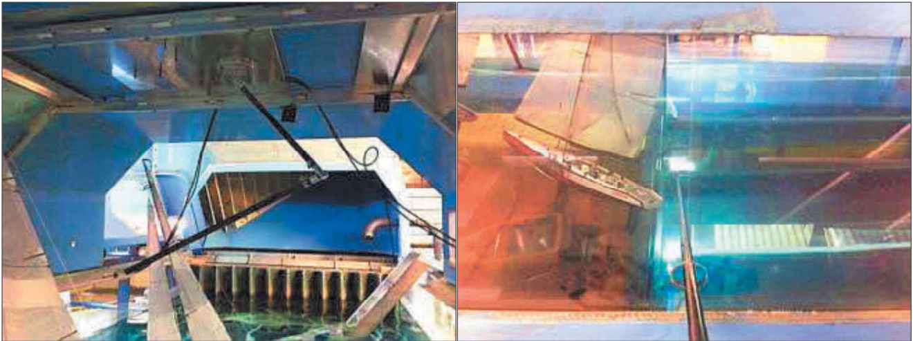
Figure 5: Fixed hot wire anemometer between the two models (left) and telescopic anemometer behind the leeward model (right)
