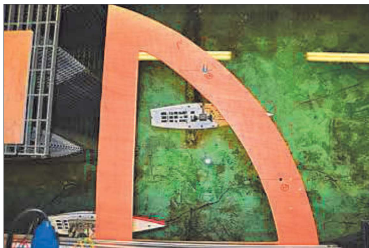
Figure 7: Plywood structure realised for Towing tank tests
