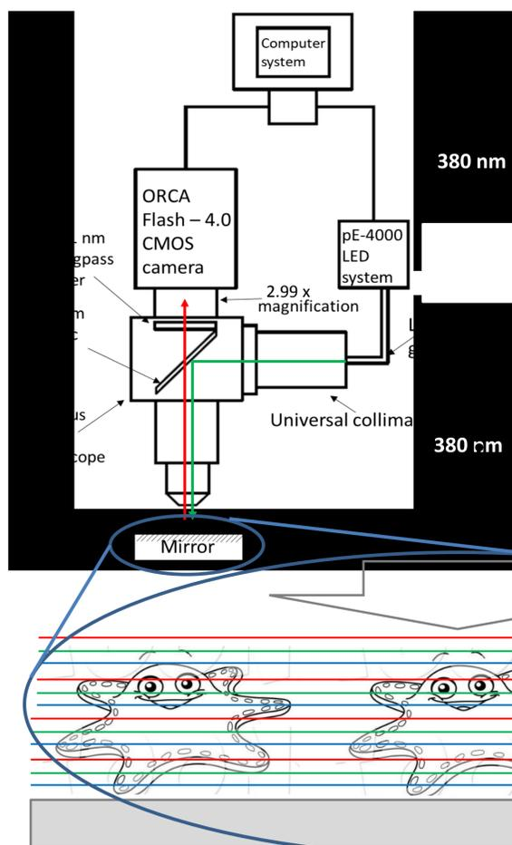
**Fig. 2:** Schematic diagram of experimental set up and demonstration of how TartanSW structure interacts with specimens.
