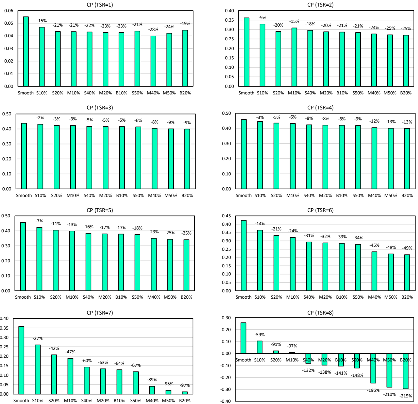
Figure 10 Comparisons of C_p values in different fouling conditions at each TSR
