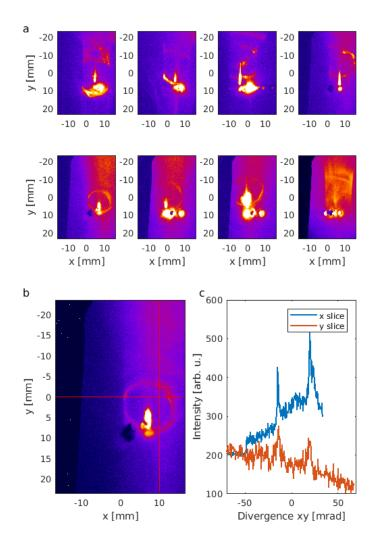
Figure 2. Electron beam profile measured on the LANEX e-profile monitor. (a) shows selected shots over a 2-day period with examples of electron ring images. (b) shows an one example with cross-sections (c) taken along the indicated lines. The ring opening full-angle in (b) is 35 mrad and the ring FWHM thickness is about 3 mrad. The full opening angle of the ring fluctuated from shot to shot between 30 and 60 mrad.
