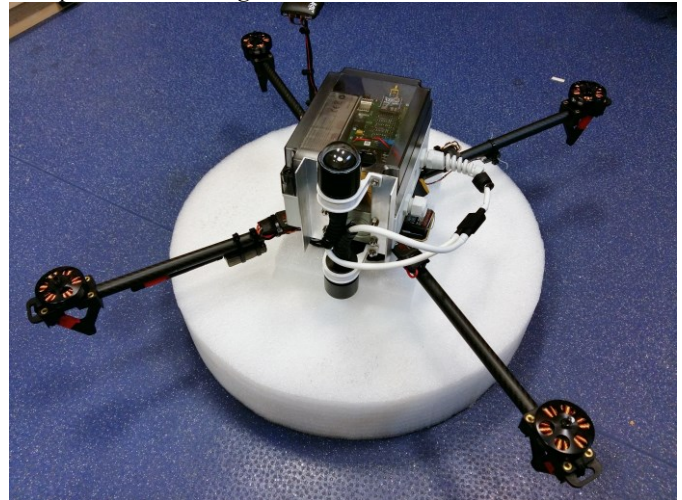
Fig. 1: Image displaying the completed integration of the IP68 housed, dual field-of-view spectrometer aboard the custom-built quadcopter system (rotary blades not included). The white polystyrene circle is for display purposes only and not part of the flying setup.
