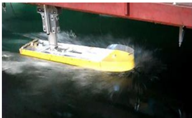
Figure 15: UNINA model experimental set up (photo at model speed V = 5.75\text{m/s} ). Adapted from Rosén et al. (2017).
