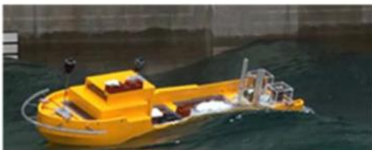
Figure 17: Free-running model experiment of the OSV in astern quartering waves. Adapted from Umeda et al. (2016a).
