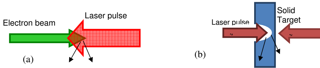
FIGURE 2. Strong field physics and QED with: (a) gas target in which the pump-laser beam generates the relativistic electron-beam which interacts with the counter-propagating probe-laser beam. (b) solid target in which the electrons are produced by the pump-laser beam and interact with the probe-laser beam or with the pump-beam itself. The pump and probe lasers are synchronized and delayed with respect to one another as required.
