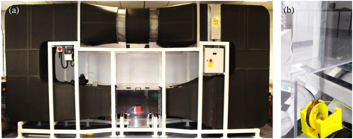
Fig. 3. (a) Side view of the closed-loop wind tunnel (b) WIFEH prototype with one coil configuration showing flutter motion at 2.3 m/s
