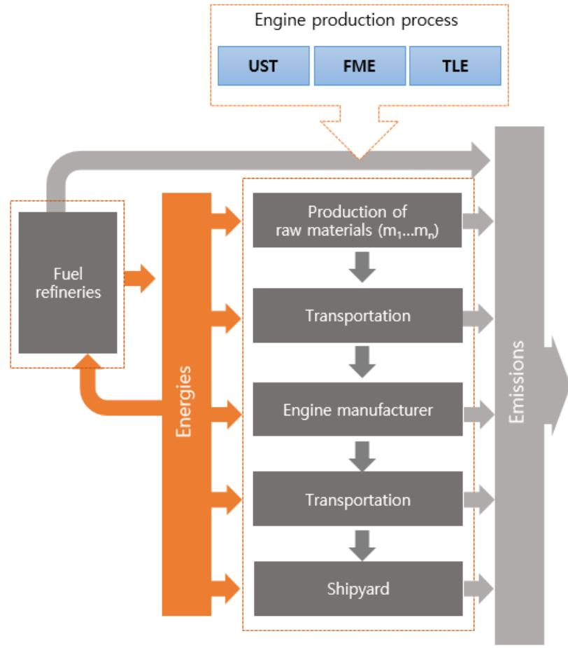
**Fig. 5.** A process of ship construction associated with engine systems.
