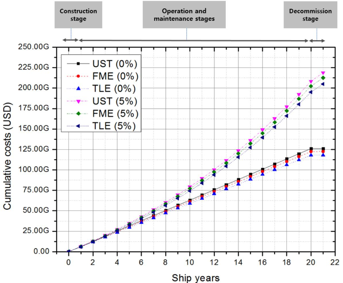
**Fig. 12.** Cumulative costs for environmental impact over ship life cycle.
