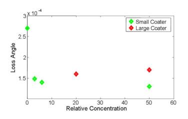
Figure 7. Plot of the coating loss angle versus the relative concentration of titania doping of tantala. The coatings were made at LMA in Lyon with two different coaters. The data show a rapid decrease of the loss with small concentrations of the dopant whereas at larger concentrations the mechanical loss seems to reach a plateau. Relative concentration expresses the fractional change of index of refraction assigning 0 and 100 to respectively pure tantala and pure titania.
