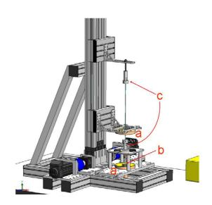
Figure 3. Rendering of the pulling machine. The configuration shown is for pulling circular fibres. The two conical mirrors "a", the rotating mirror "b" and the two clamps "c" are shown.
