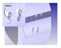
Figure 4. Rendering of two ears attached to a silica mass. The triangular shape of the ears has been designed for the reduction of the peeling effect due to the high shear stress. The height and width of the ears are respectively 25 mm and 12 mm. The fibre head is lap welded to the ear.
