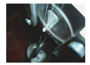
Figure 5. Top view of an ear bonded on a disk and loaded with 12 kg. The hook holding the mass is placed on the same position where the fibre head will be welded. Clock stopping wires are in place to record precisely the time of the eventual breaking.
