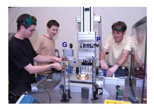
Figure 2. Picture showing the status of the  $CO_2$  pulling and welding machine. The two vertical axes are mounted whereas the horizontal one has been removed. On the machine base it is possible to see one of the gold coated conical mirrors that will be used for pulling circular fibres. As a temporary solution a mirror galvanometer mounted on a post is used to dither the laser beam for the production of silica ribbons. The periscopic system P and the galvanometer G are shown in the picture.
