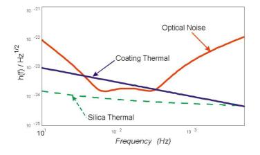
Figure 6. Square root of the power spectral density in h of some fundamental noises in Advanced LIGO. The calculation has been done with the code BENCH [22]. The mechanical loss angle used for the coatings is  $2.4 \times 10^{-4}$  [21], a value that makes the coating thermal noise the main limitation to performance at mid frequencies.
