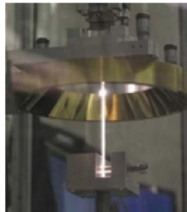
FIG. 6. (Color) The 3 mm diameter cylindrical fused silica stock being heated by the CO<sub>2</sub> laser as the fiber is pulled.
