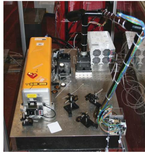
FIG. 9. (Color) The welding system consists of a CO<sub>2</sub> laser delivered through an articulated arm, ZnSe output telescope, and a pair of mirror galvanometers.
