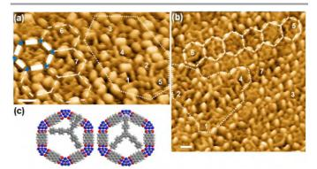
Fig. 2 High resolution STM images in 3D representation of PTCDI-melamine networks on Au(111)/mica after exposure to solutions of S-TPEB (a) and PE-TPEB (b). To guide the eye some intact cells are marked by white hexagons. Areas lacking the network structure are framed by dotted lines. Some of the S-TPEB and PE-TPEB molecules discussed in more detail in the text are labelled by numbers. (c) Models of PE-TPEB trapped in a network pore. Scale bars: 2 nm.
