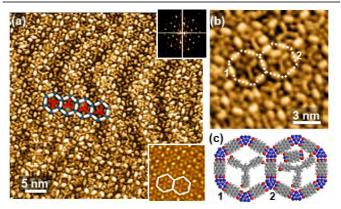
**Fig. 3** STM images of PTCDI-melamine networks onm Au(111)/mica after exposure to  $P_{OH}$ -**TPEB**. (a) As a guide to the eye a few pores with stars are highlighted. Insets show Fourier transform of image (top right) and a section of the Fourier filtered image (bottom right). (b) High resolution image with two pores marked whose structural models are shown in (c).
