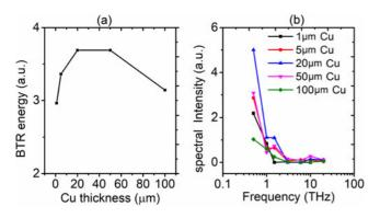
**Figure 5.** (a) The measured BTR energy as a function of copper foil target thickness. (b) The measured BTR spectrum with copper foil target thickness varying from 1  $\mu$ m to 100  $\mu$ m.
