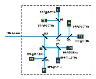
Figure 1. Schematic layout of eight-channel THz calorimeter system.
