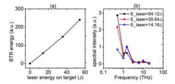
**Figure 4.** (a) The measured BTR energy from a 5  $\mu$ m copper target as a function of the pump laser energy. (b) The measured BTR spectrum with driven laser energy on target varying from 14 J to 54 J from a 5  $\mu$ m copper target.
