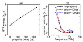
**Figure 6.** (a) The measured BTR energy from a 100  $\mu$ m copper target as a function of delay between pre-pulse and main pulse. (b) The measured BTR spectrum from a 100  $\mu$ m copper target with different delays between pre-pulse and main pulse, no pre-pulse, 400 ps and 1000 ps, respectively.
