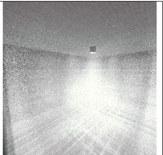
Figure 7 Non-homogeneous mist in the test room, as predicted by CFD
