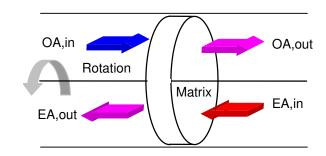
Counter-flow Heat exchanger with a correction factor
