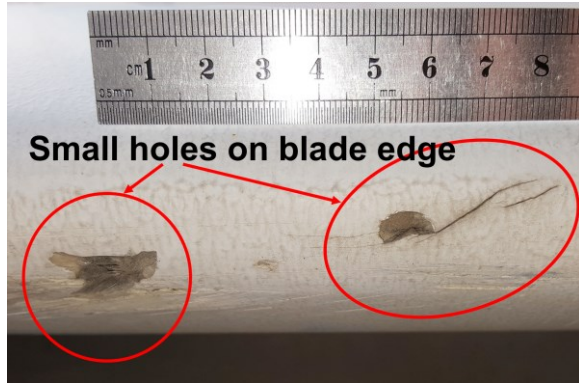
Fig. 14. Small holes are made on the leading edge in the experiments and the surface diameter of the hole is about 1cm.
