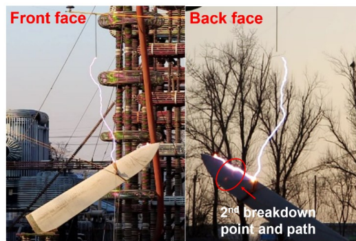
(a) Creeping discharge from receptor along the leading/trailing edge
