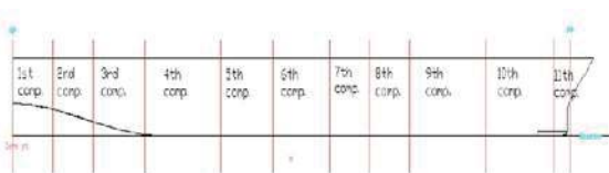
14. Figure 4 Subdivision of the frigate (Kahramanoglu, 2015)
