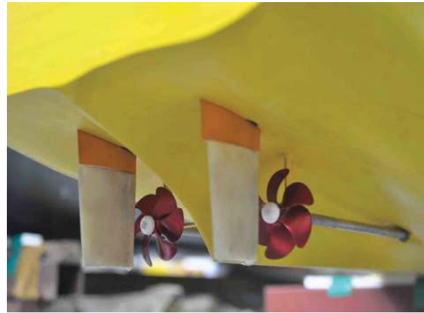
Figure 5 Fully appended stern of the test model.
