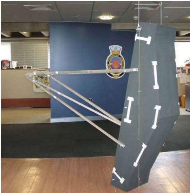
Figure 4 Establishing KG by suspension
