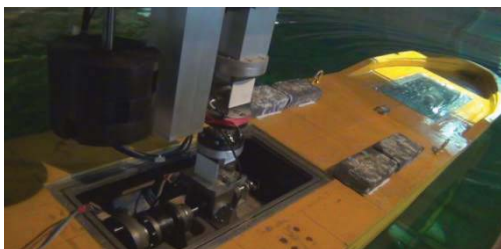
Figure 2 The ship model in partially restrained experiment
