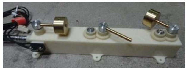
Figure 2 Forced irregular roll motion device.
