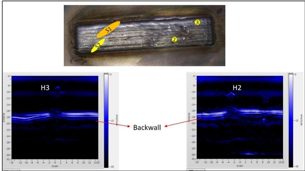
FIGURE 11. TFM (5 MHz) to detect H2 and H3
