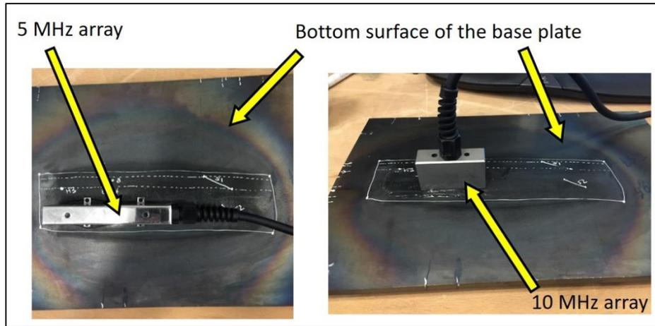
**FIGURE 7.** Phased array scanning of the bottom surface
