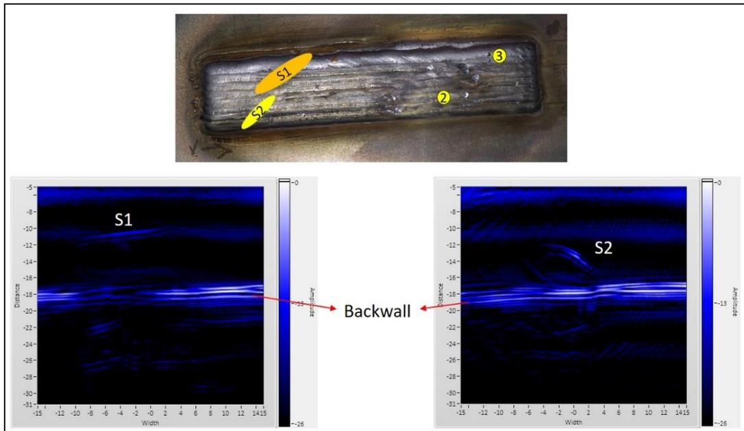
FIGURE 10. TFM (5 MHz) to detect S1 and S2
