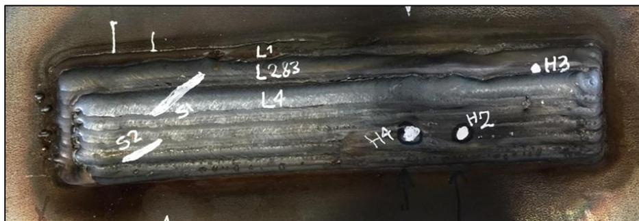
**FIGURE 6.** Defects successfully embedded inside the sample
