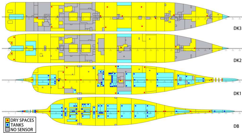
Figure 6 – Arrangement of flooding sensors according to IMO guideline.
