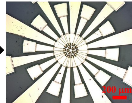
\text{SiO}_2 growth for isolation layer & Metal deposition for p-electrodes
