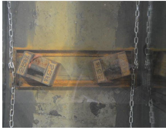
Fig. 6 A view of the chain mooring line and the iron anchor
