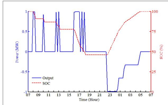
**Figure 4** Outputs (MW) of the BESS (discharge rates were positive and charge rates were negative) and corresponding variations in SOC (%) within a complete cycle from 07:00 on 03/09/2014 to 07:00 on 04/09/2014.
