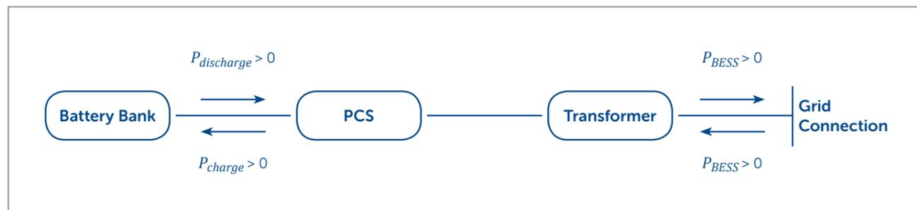
Figure 8 Simplified illustration of a BESS architecture.
