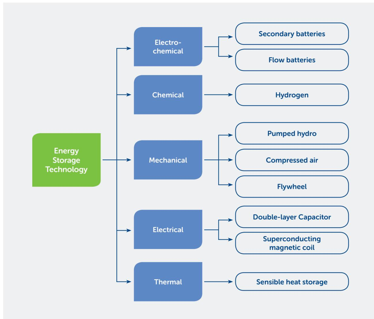
Figure 2 Classifications of energy storage technologies [1].
